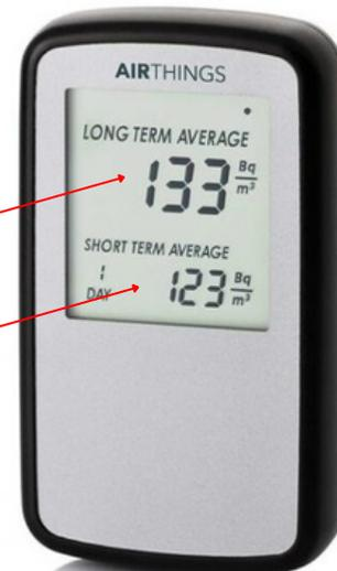
The radon screening device in this kit is called a Corentium Home, by Airthings. It is an electronic device that measures radon.
